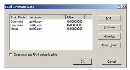
Figure 5.97 Load Coverage Data dialog box
